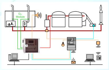
The fundamental information for optimum operating management both for gas production and for gas recovery (cogeneration units and burners) are given by the measurement of the raw gas composition ( $CO_4$ ,  $CO_2$ ,  $O_2$ ,  $CO_3$ ). Information about H<sub>2</sub>S concentration enables the preventive measures to avoid damages in gas fittings, cogeneration units and boilers.
